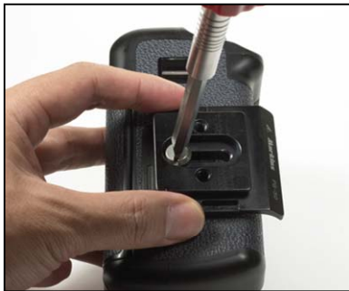
4. Screw in but not tighten the bolt to the body while leaving one or two turns.
