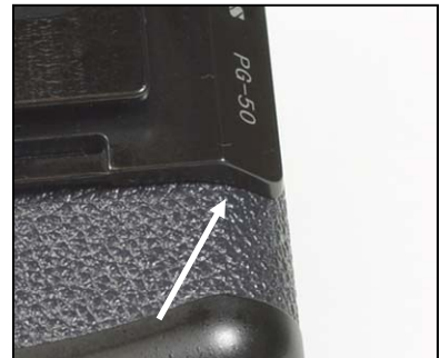
6. Make sure that there is no gap between the flange and the camera body.
