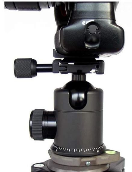
Screw the plate tight. Newest plates are shipped with an improved hexagonal head cavity screw for a 5/32" Allen wrench for positive locking.
