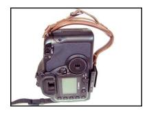
Loosely attach the plate, and adjust the strap to fit your hand. And, tighten the plate.
