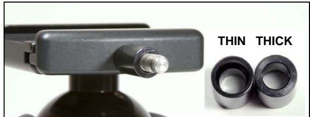
4. Insert the new spacer. (Thick walled side faces the knob.) The new spacer is shorter than the old one in length.
