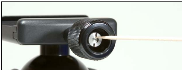
7. Apply a small drop of superglue to the seam between the stopper and the shaft using a sharp object such as toothpick. This will prevent the stopper from loosening by vibration and usage.
